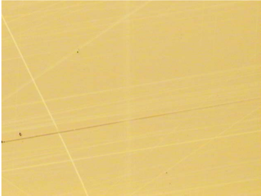
Figure 5 : Damage under 1N during progressive scratch
