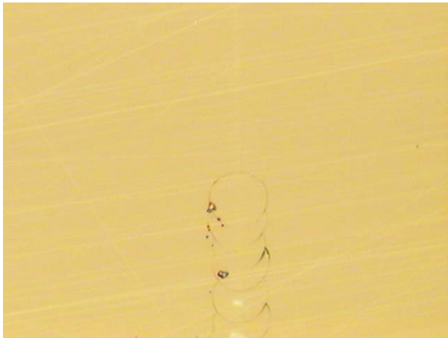
Figure 6 : First circular crack during progressive scratch
