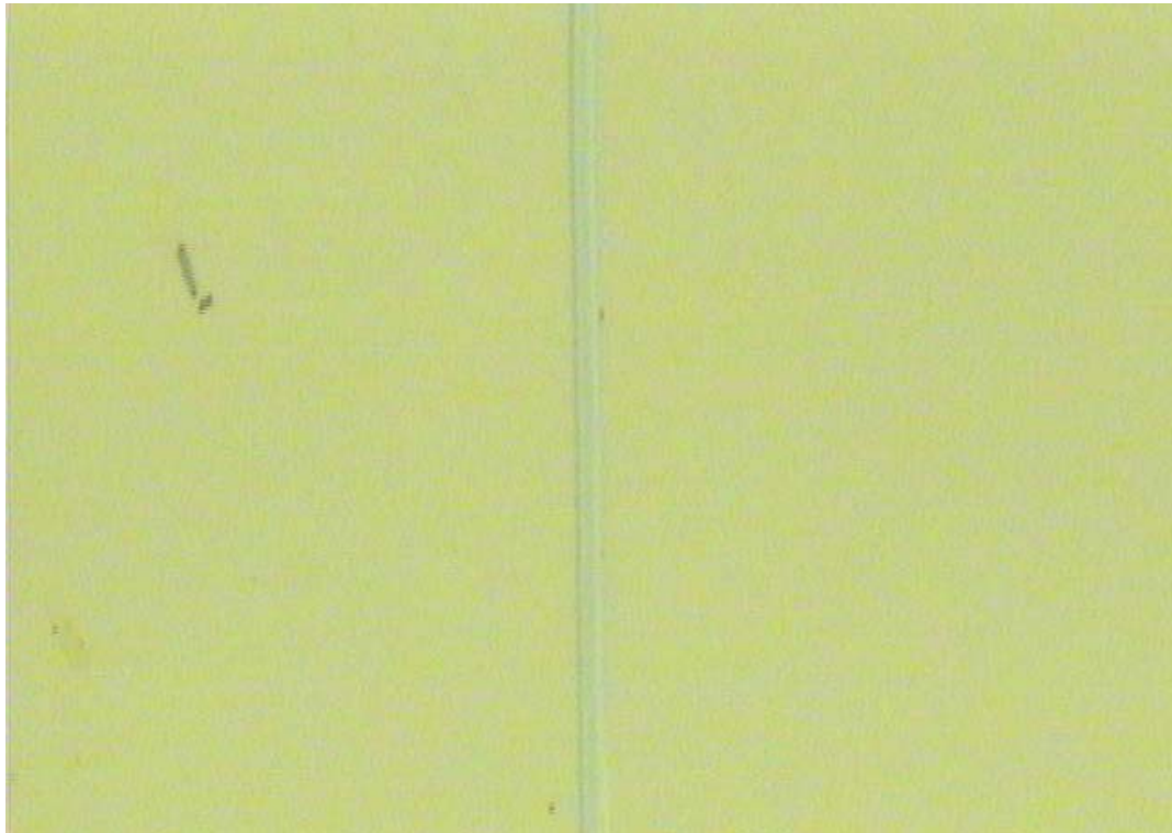
Figure 7 : Micrograph of the Scratch at Failure – SiN on Glass 500x magnification (image width 0.0615mm)
