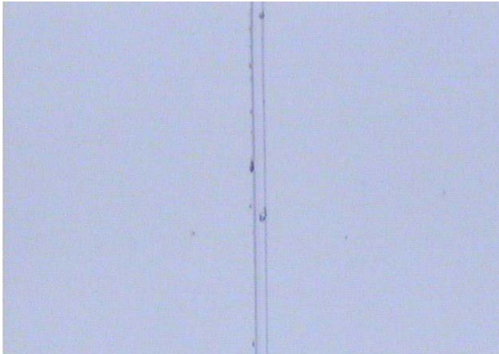
Figure 2 : Micrograph of the Scratch at 20 mN – Al on Glass 500x magnification (image width 0.0615mm)
