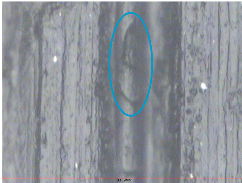
Micrograph of Initial Damage – SAMPLE 2, Scratch 3 500x magnification (image width 0.102mm)
