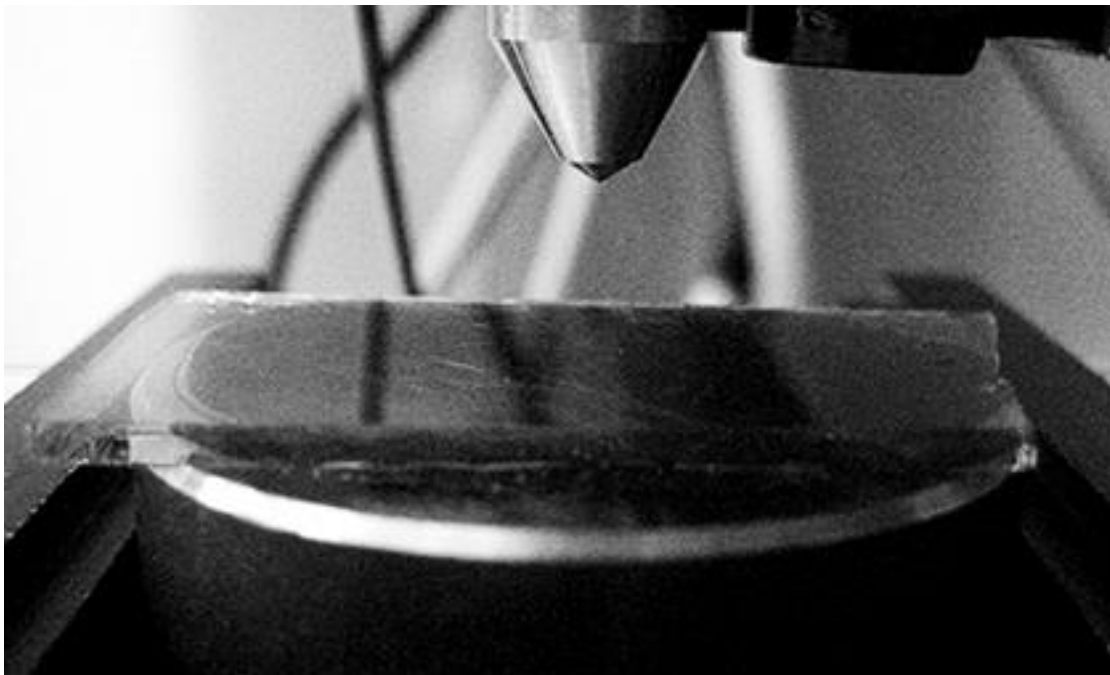
Fig. 1: Micro indenter on the glass sample.
